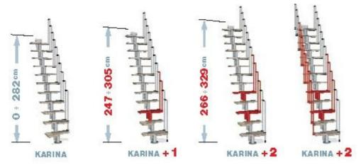
The standard staircase kit always starts with a left-footed tread. Once you add risers, the installation starts with a right-footed tread (see drawing above).
